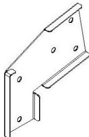
A4M00511 | VIGA DEL COLUMPIO EXTERNA SOPORTE IZQUIERDO COLOR AZUL
